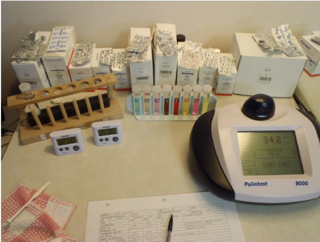
Figure 4. Photo showing a typical set-up for photometer analysis. Reagents are in silver packaging aligned atop. Coloured sample solutions ready for analyses are shown in the 10 ml tubes in rack. The Photometer is in the lower right of the photo.
