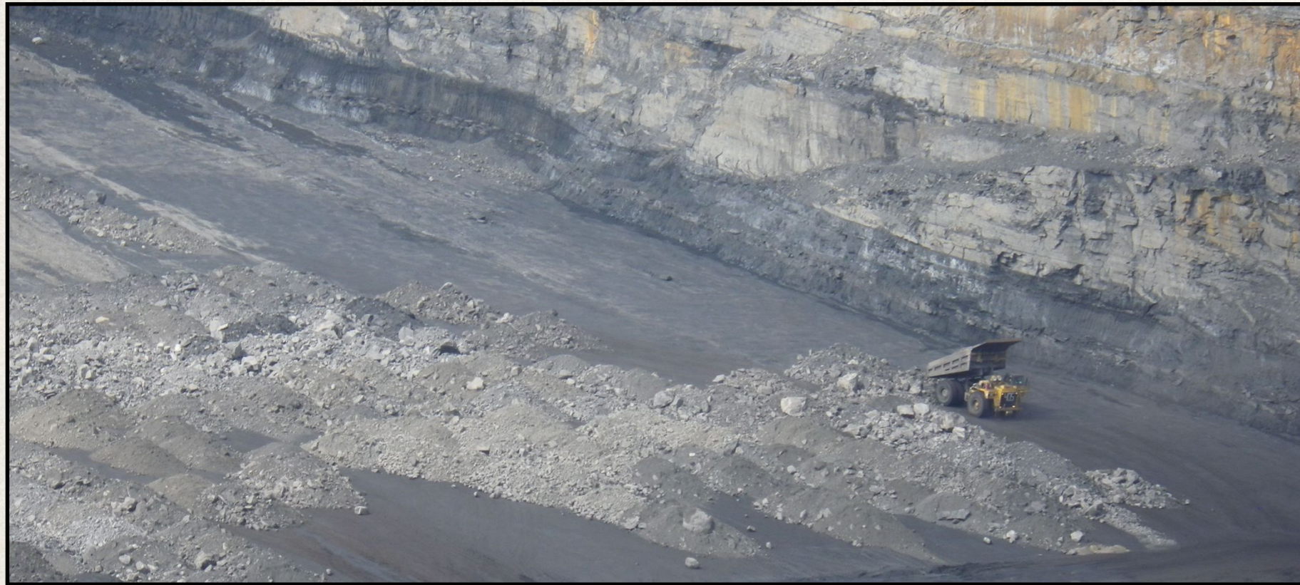
Dumping waste in mined-out area, “J” seam in background
