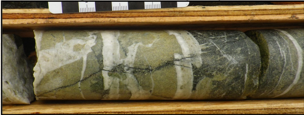
18-1096: complex quartz-magnetite vein in sericite schist, Mitzi prospect
