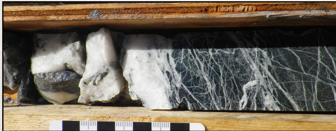
SB-18-03: 45m, quartz vein and stockwork
