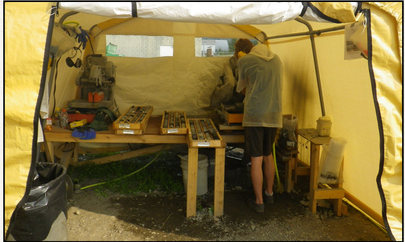
Sawing core, Fran project
